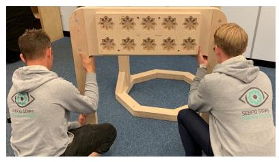
Lift the Mounting Board / Straight Uprights section onto the base section.
