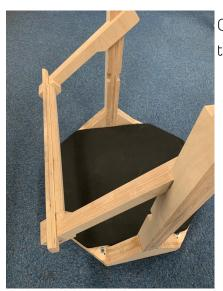
Once the Portal Foot struts are installed, slide the bar into place.
