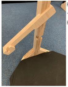
Place the Portal Foot struts in a notch on the Upright.
